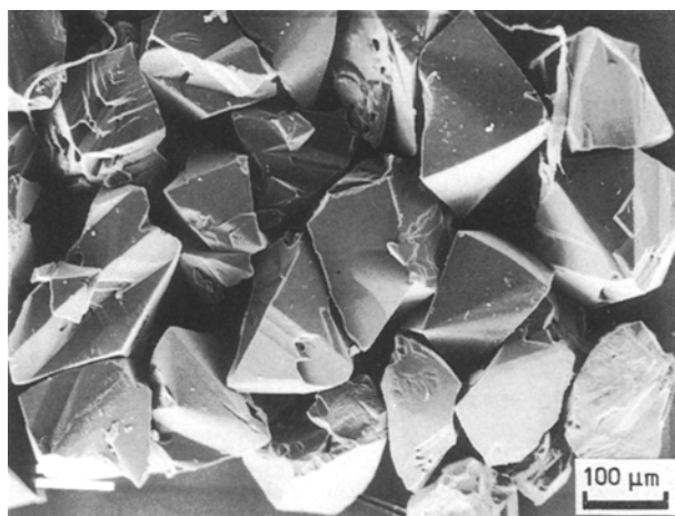
Figure 5 SEM micrograph of cubic BN crystals grown from the system \text{Li}_3\text{N-BN} .
